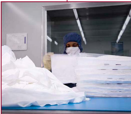
Photo A – ISO Class 5 Production Cleanroom
